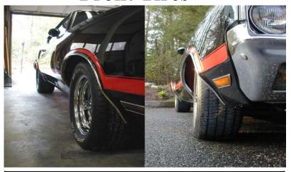
On the left is the new rubber, P265-50R15's on  $15 \times 8$ " wide rims, on the right are the old P245-50R14's . When going this wide in the front, extra care is required to make sure the tires do not rub the suspension or frame when turning at both full compression and full extension. These fit well and I have not see any rubbing at all.
